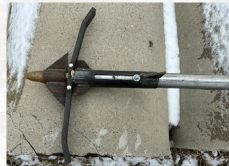
The Grapple Hook Culvert Cleaner, fabricated with shop scrap metal, has a 1.65-inch diameter hook useful in pipes of at least 24 inches.
