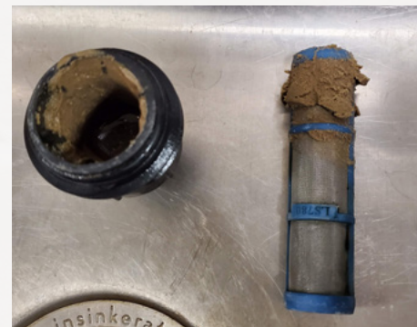
Filters clogged during the brine production process because ordinary road salt contains a lot of grit and fine particles.
