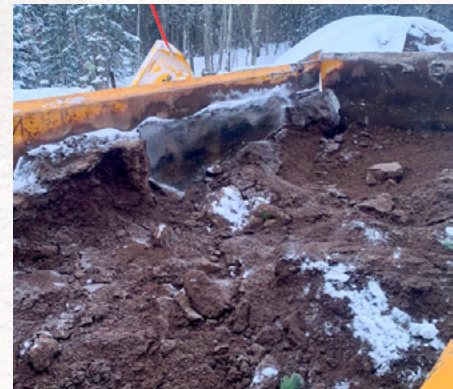
Clumps of frozen sand treated with potassium acetate formed when temperatures fell below zero.
