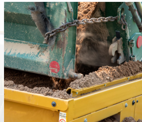
Design improvements prevent the tailgate pin of a gravel supply truck from snagging on the frame of the road shouldering machine.
