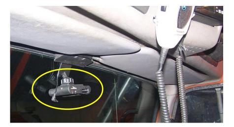
Figure 7: GPS dash camera for recording snowplow runs
