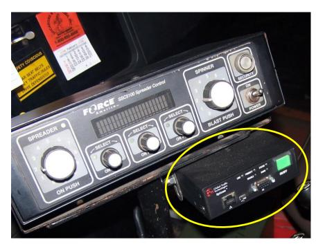
The second piece of equipment is the GPS preemption unit and control panel that allows the operator to turn the GPS preemption system off and on. A small cable runs between the antenna and the control panel. See figure 6.
