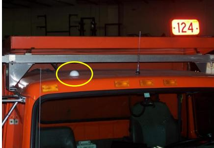
Figure 5: GPS receiver and communicator antenna
