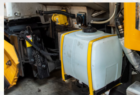
Installation of the nurse tank system costs approximately $1,778 per truck in labor and materials.
