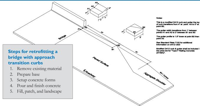
So far, Jackson County has retrofitted two bridges with the approach transition curb. The county plans eventually to retrofit all bridges on paved roadways, prioritized by worst condition first. Public works staff continue to monitor the performance of the improvements for any needed adjustments.
