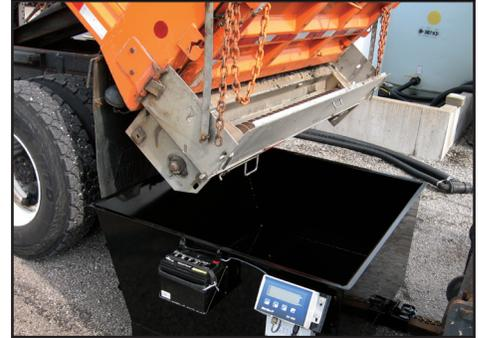
**Problem** During the winter months, Olmsted County uses 17 tandem-axle snowplow trucks to maintain 530 miles of roadway. The county was unable to verify the amount of salt and sand being applied to the roadway by these vehicles because it lacked a uniform method for calibrating the sanders on each truck. It was difficult to determine if the amount of salt and sand applied was sufficient or if the county was overspreading the material.
