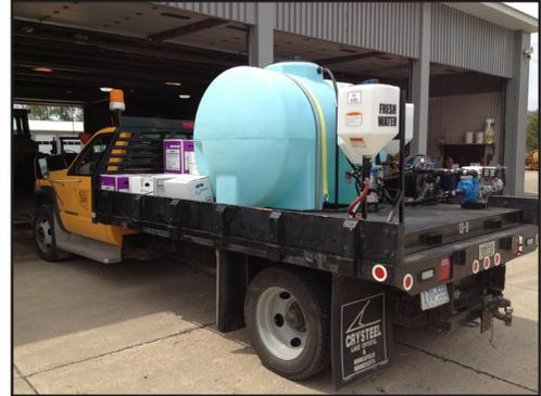
**Solution** The county designed and fabricated a versatile spraying unit. The unit consists of a mountable platform that contains tanks, hoses, and a pump, which can be easily installed on and removed from an existing flatbed one-ton county pickup truck. The unit can spray multiple chemicals at once while keeping the chemicals away from the applicator. It can also be tracked by GPS to assist in year-to-year documentation and in any crop damage claims.
