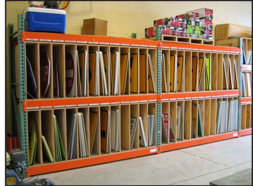
**Problem** Olmsted County lacked the ability to efficiently store and maintain its sign inventory. Signs were stacked and stored in locations that were unorganized and not easily accessible, such as on metal racks. Due to the high cost of signs that have either diamond grade or high-intensity sheeting, a more efficient means of storing, organizing, and maintaining the inventory was needed to prevent damage.
